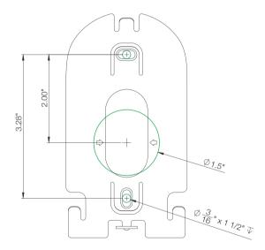
Prepare holes using mounting plate as a template and drill.
