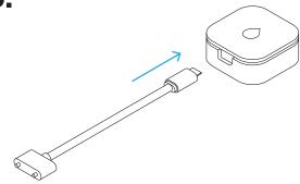
If mounting the Latch Water Sensor on the wall, connect the external extension probe. Remove the waterproof plug that covers the USB interface and connect the extension water probe into the device terminal.
