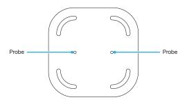
If deploying the Latch Water Sensor on the ground, probes should face the floor.
