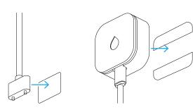
In order for the sensor to work, both probes must have contact with water. Attach probes to a clean, dry surface using adhesive pad.
