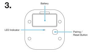
Note: If a network is not found after 100 seconds, the sensor will go into sleep mode. To wake the sensor again, press the pairing button once to trigger the pairing process
