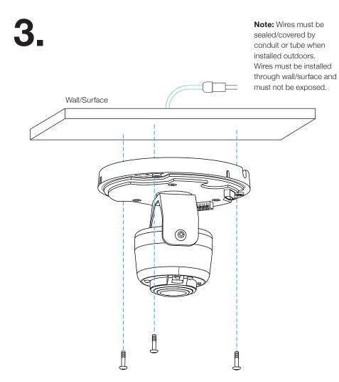
Please ensure the Mini Dome Camera is configured and added to the network before mounting.
