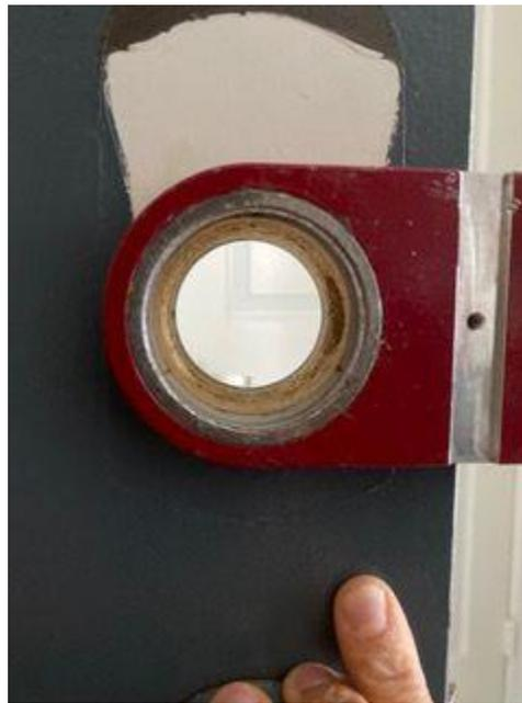
1. *Example of Door Knob/Lock Installation Jig*
