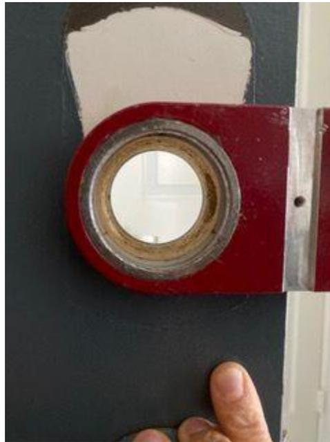
*Example of Door Knob/Lock Installation Jig*
