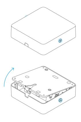
Rotate Torx screws in outer Cover counter-clockwise to unlock. Separate the outer Cover from the Mounting Plate using the opening on the underside.
