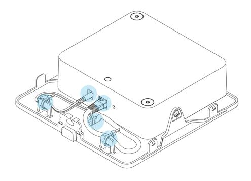
Plug in power and Ethernet cables. Use included cable ties to secure. Install Grommet.
