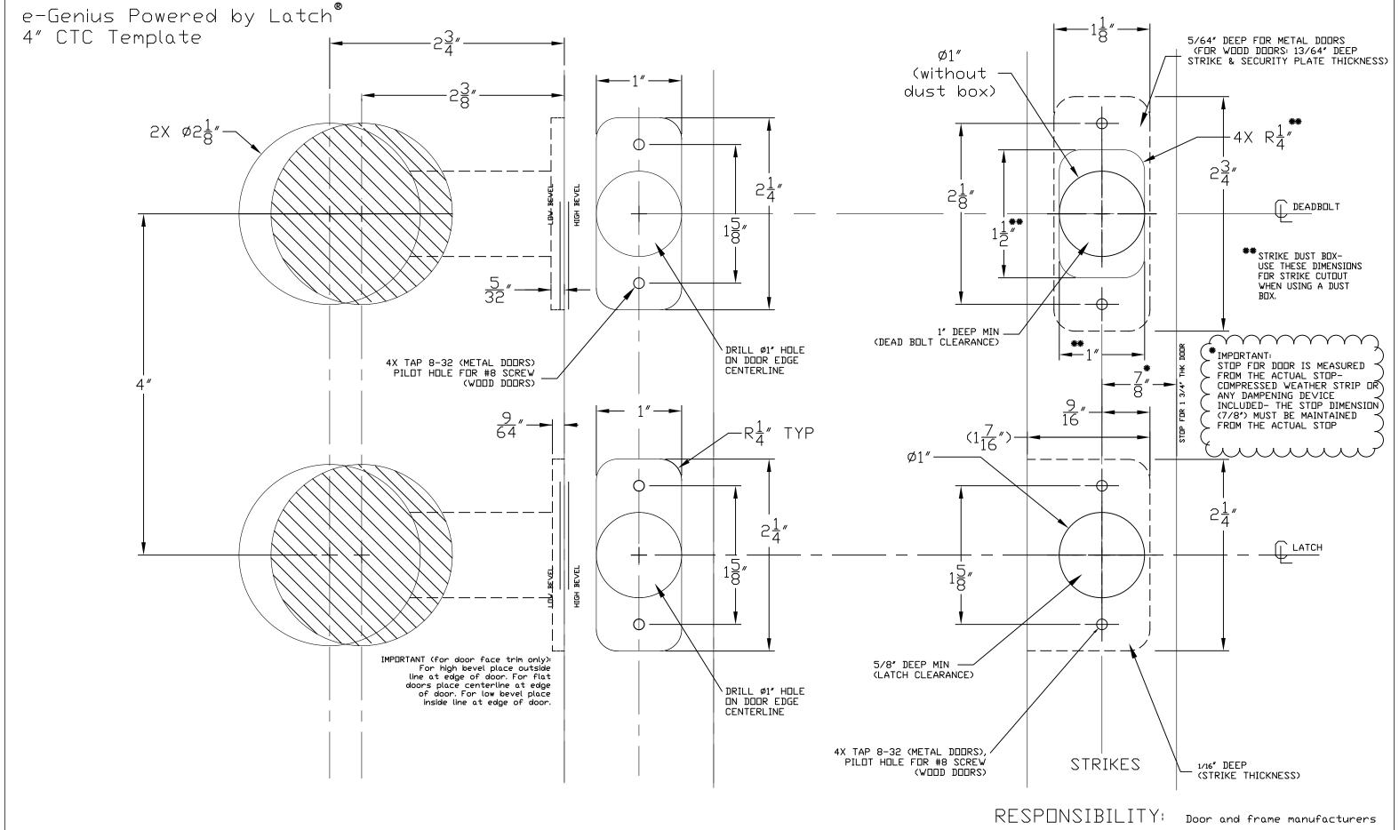
ESPONSIBILITY: Door and frame manufacturers are responsible for providing adequate construction or reinforcements for proper installation of hardware.
